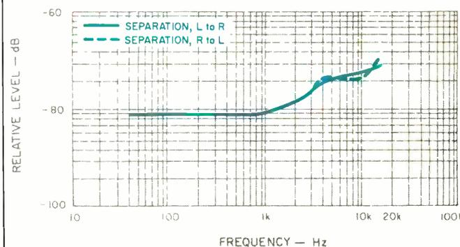
Fig. 5—Separation vs. frequency, from left to right and from right to left channels.
