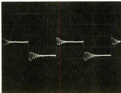
**Fig. 2—Square-wave response. Test record is CBS CTC-310.**
