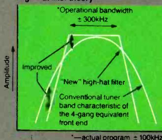
The SST circuitry also solves the problem of front end tracking error, which occurs when the center of the bandpass filter is not at the exact frequency of the broadcast signal. SST eliminates such error by using separate control
