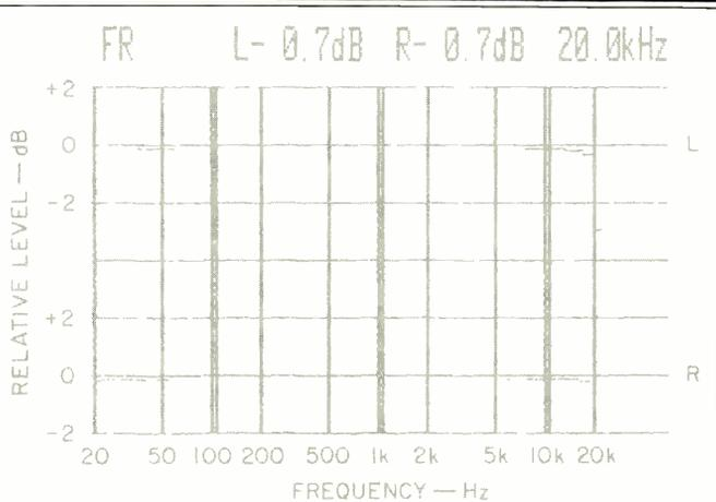
**Fig. 1—Frequency response, left (top) and right channels.**
