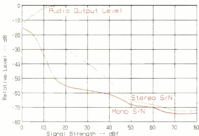
**Fig. 1—Mono and stereo quieting characteristics, FM section.**
