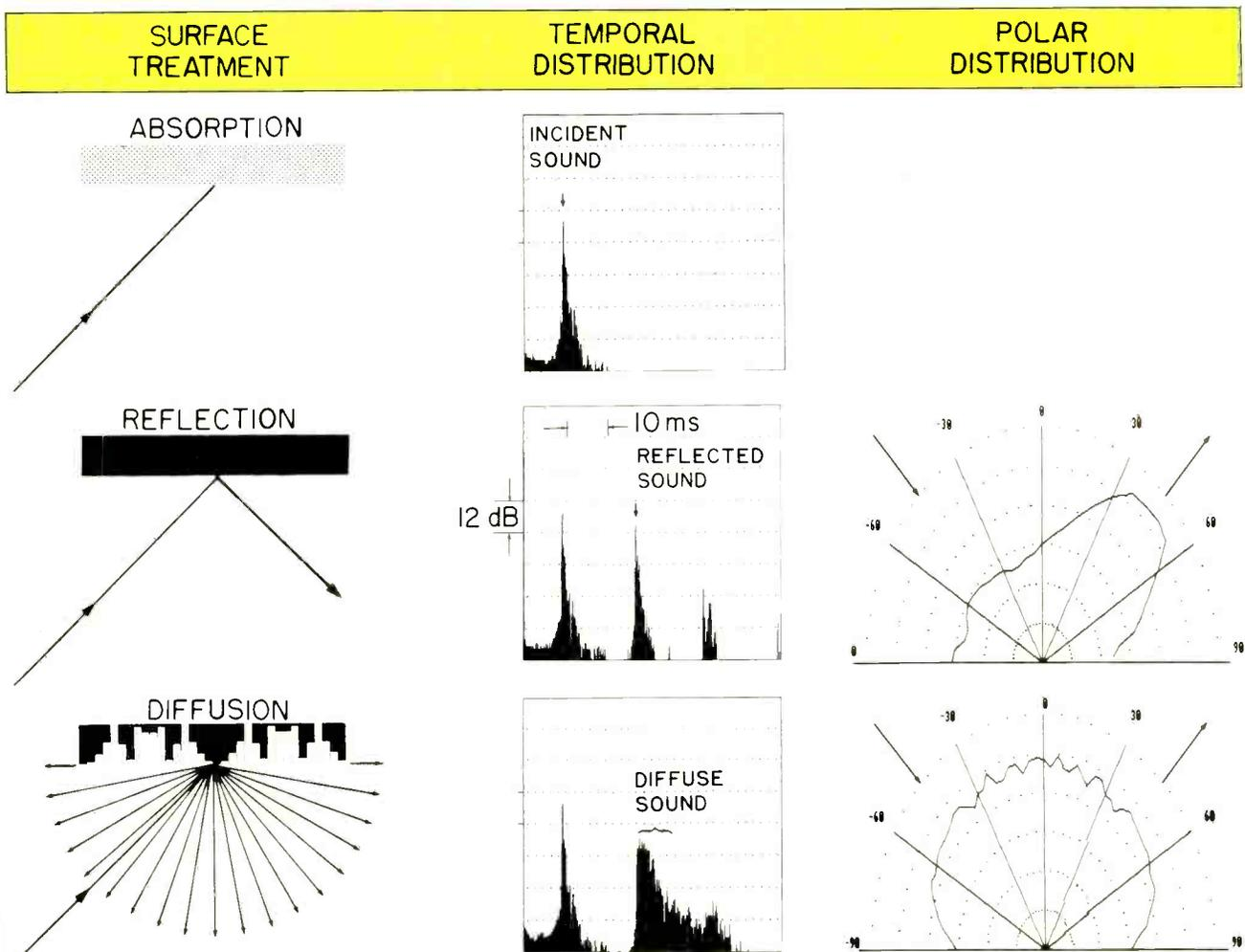
Fig. 2—Comparison of temporal (time) and spatial (polar) diffusing properties of absorptive, reflective, and diffusive surfaces. The scattered energy from an ideal absorptive surface (top row) is negligible; therefore, no polar plot is depicted. The energy scattered from a reflective surface
