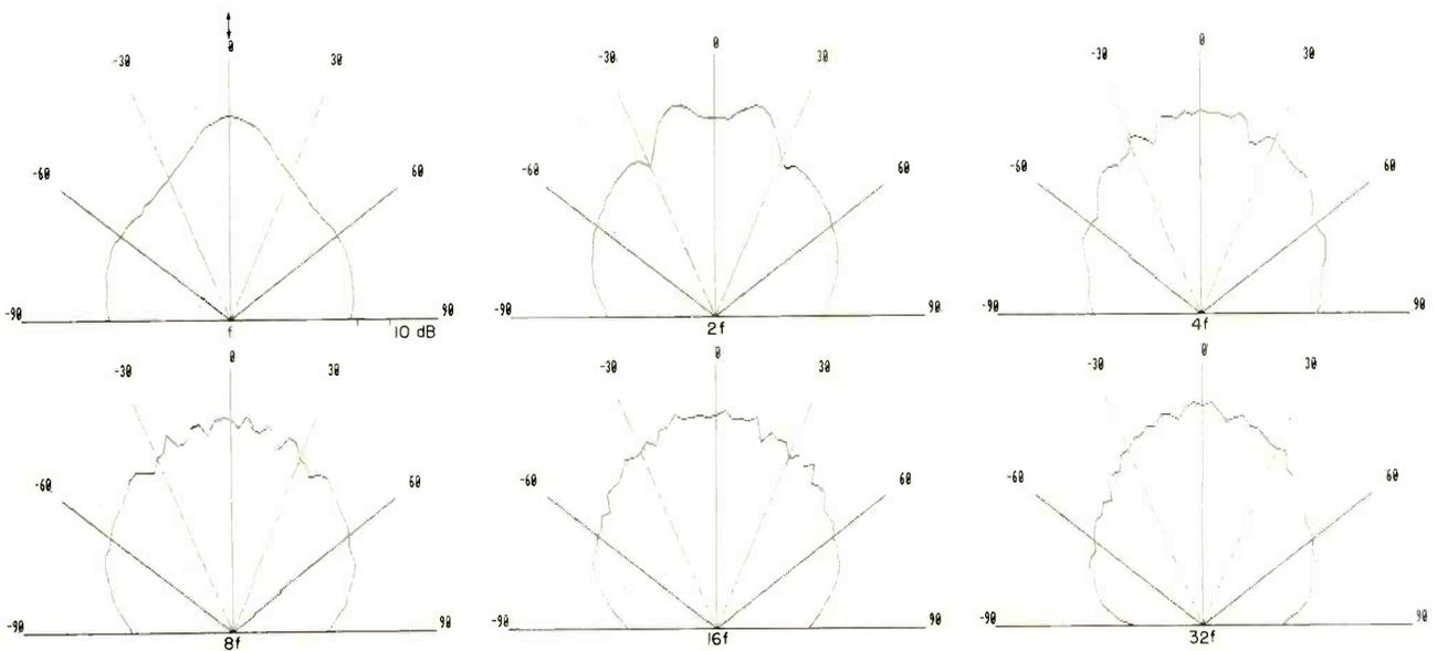
Fig. 4—Polar energy response from an RPG diffusor, showing uniform scattering between  $-90^\circ$  and  $+90^\circ$  over five musical octaves from  $f = 250$  Hz to  $32f = 8,000$  Hz.
