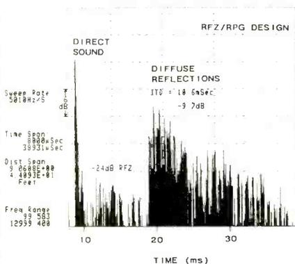
Fig. 8B—Energy-time curve of Pisha's listening room of Figs. 6 and 7 after RFZ/RPG treatment, showing much improved response. An initial time-delay gap of 10 mS was created with an RFZ 24 dB below the direct sound. The reflection pattern consists of a dense, uniform, exponentially decaying sound field.
