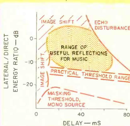
Fig. 1—The effect of delayed reflections of various intensities on the perception of music. (After Barron.)
