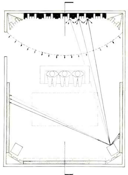
Fig. 5B—Side view of same room as in Fig. 5A, showing absorption on side walls, vertical Abffusors from floor to ceiling in front corners, and absorptive treatment on ceiling. For greater spaciousness, a diffusive ceiling can be used, in which case upper side walls reflect laterally diffused sound (dashed line with arrow) from ceiling diffusors.
