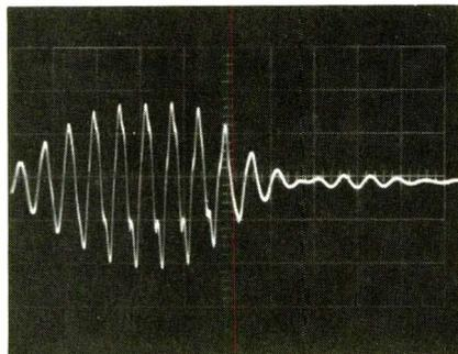
**Fig. 3—Output for 10.8-kHz pulse test at 30 cm/S, a very high recorded level. Test record is Shure TTR-103.**
