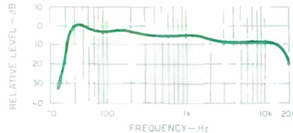
Fig. 8—Peak-level spectral envelope for overtures (CDs 15, 21, 23, and 24) and Stravinsky's "Firebird" Suite (CD 14).
