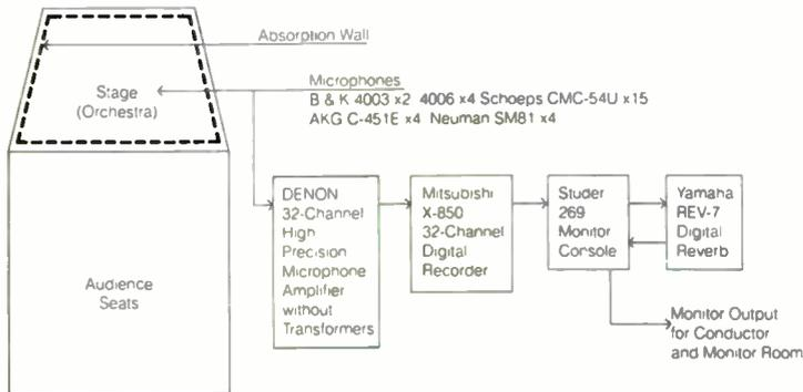
Fig. 2—Setup for Denon's anechoic recording.
