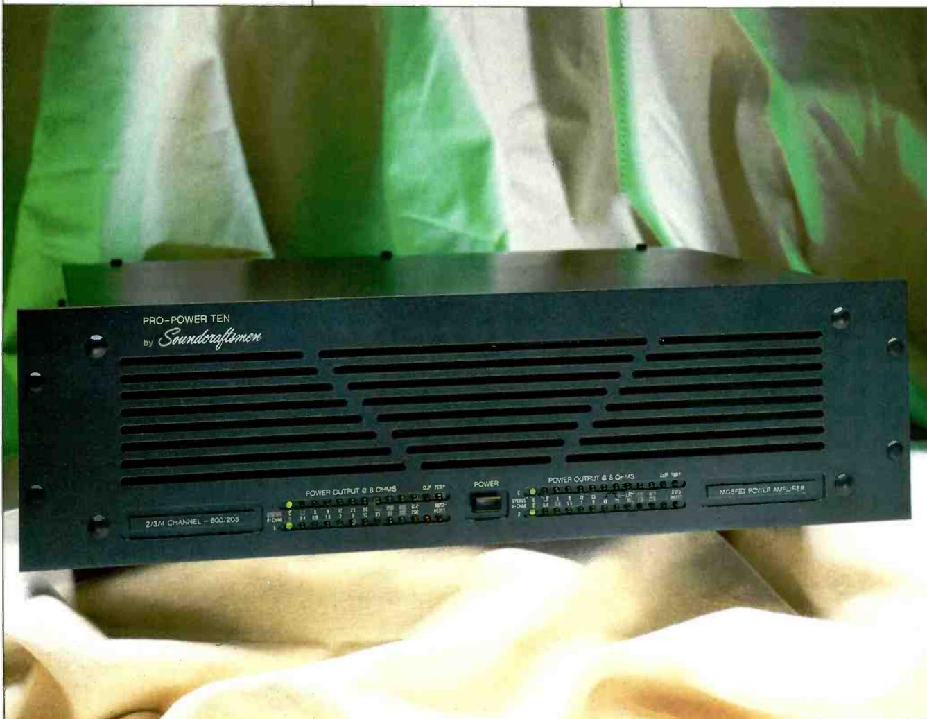
This new amplifier from Soundcraftsmen uses Class AB MOS-FET power output stages and the manufacturer's phase-controlled power supplies. Soundcraftsmen chose to use a rather stiff power supply—one that adjusts its supply voltage to match the demands of the loudspeaker. Thus, you won't find much "dynamic headroom" in this amplifier—but then again, you won't need much, in view of this unit's continuous power rating.
