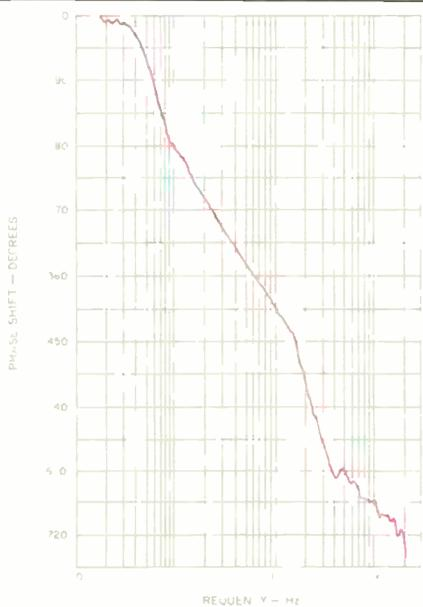
**Fig. 5—**One-meter on-axis anechoic phase response.
