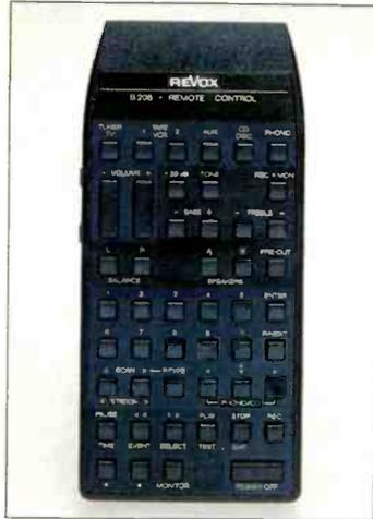
Because it also controls other Revox components, the B208 remote unit has more buttons than the B215 tape deck.
