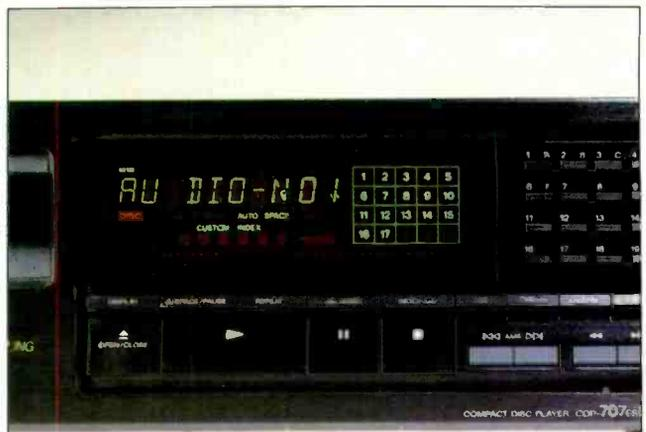
"Disc Memo" allows you to assign a message of up to 10 characters to each CD; every time a disc is loaded, its "memo" is displayed on the player's front panel.
