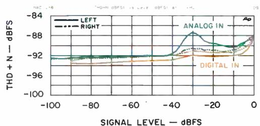
**Fig. 4—THD + N vs. level at 1 kHz.**
