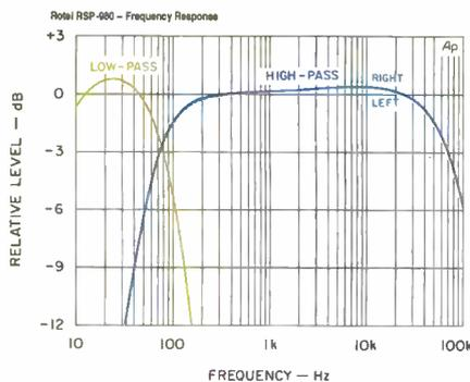
**Fig. 1—Frequency and crossover response of RSP-980 in stereo mode.**
