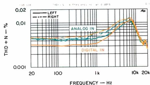
**Fig. 3—THD + N vs. frequency at 0 dBFS.**
