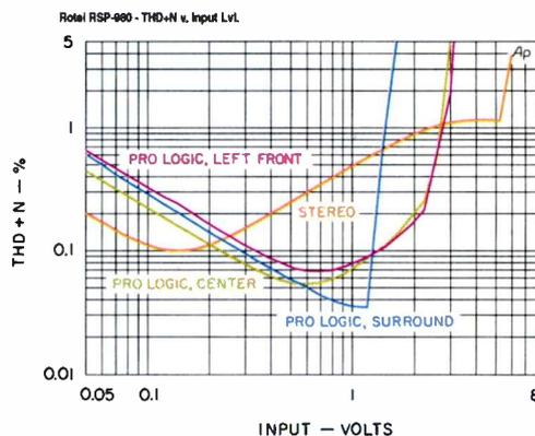
**Fig. 4—THD + N vs. input voltage, RSP-980.**
