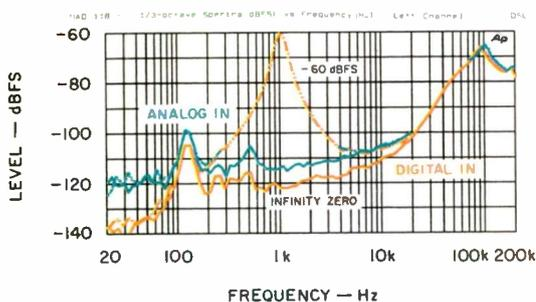
Fig. 7—Spectrum analyses for “infinity zero” signals and 1-kHz tones at -60 dBFS.
