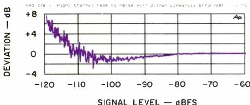
Fig. 6—Fade-to-noise test.
