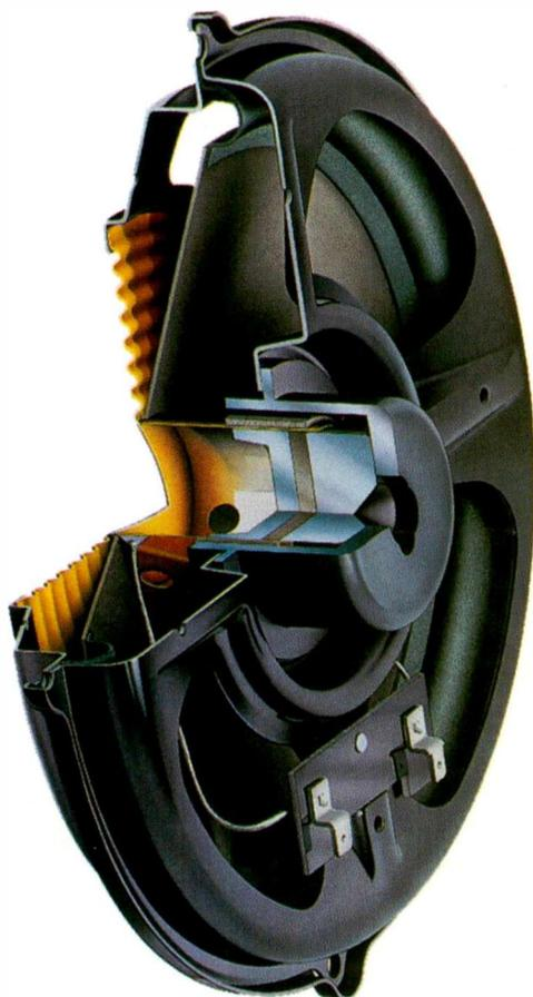
**B**ose slimmed its Nd woofer (above) by putting the magnet out front; Infinity's Kappa UniPlanes (middle right) were slimmed by turning their cones inside out.
