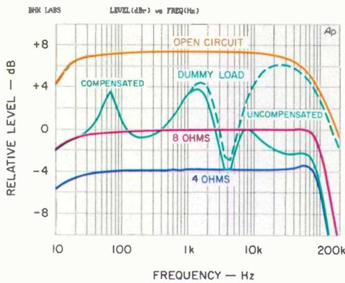
**Fig. 1—Frequency response as a function of loading.**
