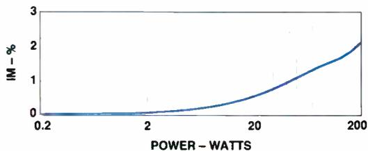
**Fig. 8—IM distortion for  $A_4$  (440 Hz) and  $E_1$  (41.2 Hz).**
