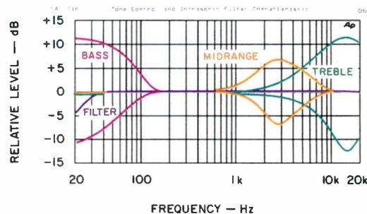
**Fig. 2—Tone control and infrasonic filter characteristics.**
