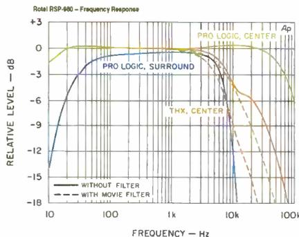
**Fig. 2—Center- and surround-channel responses, RSP-980. For clarity, surround-channel curve has been lowered by 0.5 dB.**
