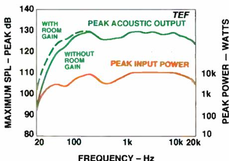
**Fig. 9—Maximum peak input power and sound output.**
