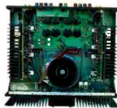
RB985 interior shown with massive power supply and select grade components. 5 x 110 watts per channel into 8 ohms.
