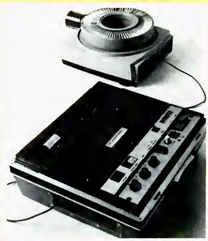
● The cassette transport is a heavy-duty a.c. powered cassette recorder/player. Narration and sync signals are recorded either independently or simultaneously. The sync signals are designed to trigger slide projectors. The model 2550 uses a 60-Hz signal to activate the tripping mechanism. However, the recorder will reliably sense slide-change signals from 50 to 2000 Hz where the sync signal pulses and audio program are recorded on two separate tracks.
