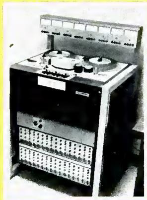
The new Pro 72 uses one-inch tape and records 8-track. There is sel-sync and plug-in modules.
