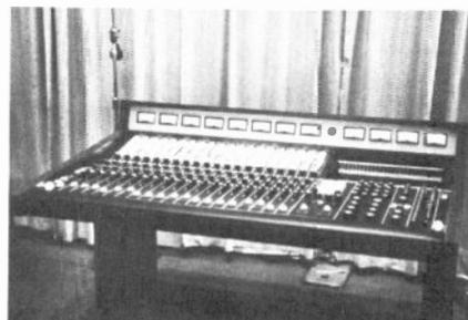
The **Spectra-Sonics** console has 20 channels in for 8 channels out. *Circle 88 on Reader Service Card.*
