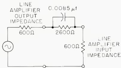
**Figure 3.** This complementary boost circuit will give you the correction shown in Figure 2 if it is inserted between line amplifiers.
