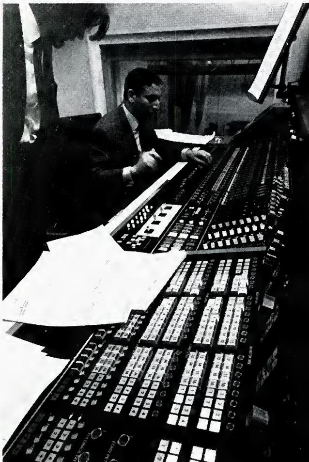
New sixteen-track recorders are essentially limited in performance by tape noise. No matter what tape is used, noise increases by about 9 dB when the sixteen-track original is mixed down to a two-channel stereo master. This is equivalent to cutting track width down to that of an 8-track cartridge and reducing tape speed to  $7\frac{1}{2}$  ips. What a waste of time, money, and effort.
