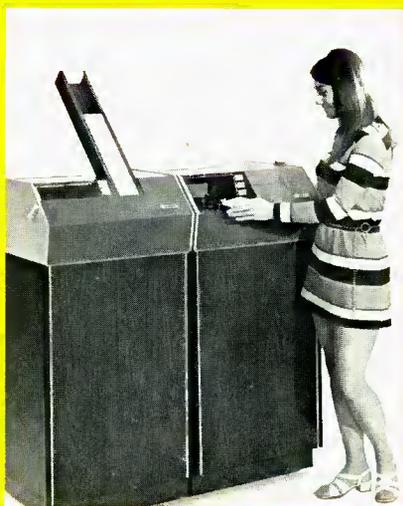
slave units. The tape is pulled out of the cassette into the vacuum chambers where the duplication process occurs. This results in close tape-to-head contact and assures gentle, precise tape handling despite the high tape speed. In addition, solid-state broadband electronics are used in the system to
