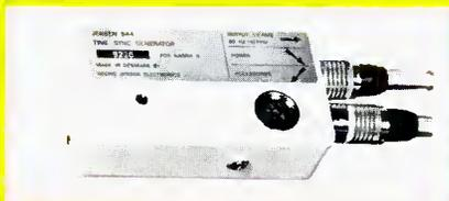
• A crystal time-sync generator for synchronizing a camera with the Nagra III or IV or Tandberg Model 11-1-P is now available. It is powered by the recorder and produces a 1.0 volt, 60 Hz synchronizing signal, with an accuracy of better than 10 parts per million which is less than  $+1/6$  frame in ten minutes. The synchronizing signal is recorded on the tape by the Neo-Pilot System, along with the audio signal.
