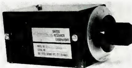
•A line of inexpensive dip filters is now offered with dip attenuation variable in 2 dB steps with a maximum of 10 dB attenuation. Dip frequencies offered are 3-5-7 kHz. A 14 kHz sync filter model will attenuate the 14 kHz sync signal greater than 45 dB. All filters are 600-ohm and have a 1.5 dB insertion loss. Tolerance is 1 dB non-accumulative. A plotted curve, knob, and dial plate is provided.
