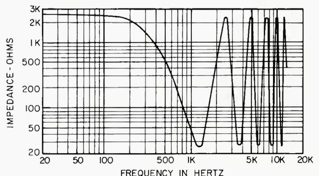
**Figure 3.** The reason for classic matching—and when it is important, when the input terminates as considerable length of line. Here is the impedance reflected to the sending end, when a line with characteristic impedance of 250 ohms, and a transmission time of 200 microseconds, is terminated with 2.5 k, the value presented by circuit in Fig. 2 (B).
