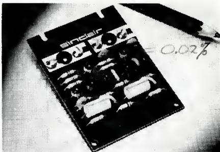
•The model Z 30 is a complete power amplifier employing 9 silicon epitaxial planar transistors. Total harmonic distortion is only 0.02 per cent at full output. Power output is 15 watts continuous into 8 ohms using a 35-volt supply. Input sensitivity is 250 mV into 100k ohms and output impedance is 3-15 ohms. The amplifier may be powered from any supply delivering d.c. over an 8 to 35 volt range. A 35-volt supply model PZ6 is available.
