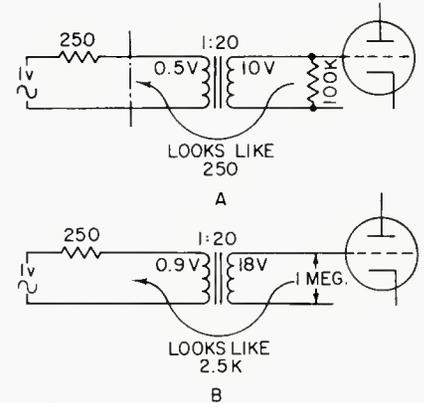
**Figure 2.** Use of an input transformer in a tube amplifier: (A) using the idealized classic matching, through the transformer; (B) using only the input impedance of the grid circuit. The latter results in a voltage gain of somewhat less than 6 dB.
