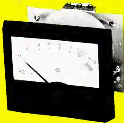
● The M-900 is a relatively inexpensive peak reading meter with a linear dB scale from +9 to -36 dB. It makes possible an ability to operate close to the overload level without creating distortion. Important specifications include: voltage requirement is 24 V d.c.; current consumption is approximately 20 mA; input impedance is 10 k ohms unbalanced; indication linearity is  $\pm 1$  dB; integration time is approximately 10 ms; and fall back time is 2 seconds full scale (adjustable).
