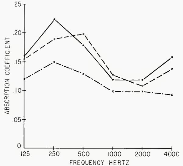
FIG. 3. Absorption characteristics of various plywood splays.
