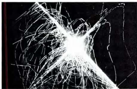
● The Technics by Panasonic people have been demonstrating quad to consumers with a large screen four-channel vectorscope made from a color c.r.t. that has been mis-converged. The resultant display was photographed for us by them to illustrate this special four channel issue.
