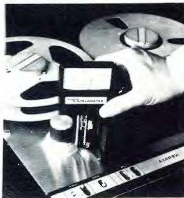
The Tentel tape tension gage is designed to diagnose problems in your magnetic tape equipment. Throw away your fish scales (or put them in your tackle box where they belong). The TENTELOMETER will measure tape tension while your transport is in operation, so you can "see" how your transport is handling your tape . . . smooth, proper tension for quality recording? or oscillating high or low tensions causing pitch problems, wow and flutter?
