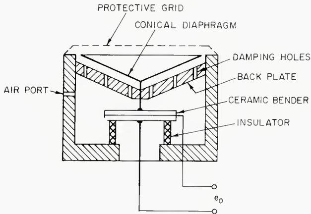
Figure 4. Schematic construction of a ceramic microphone.
