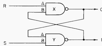
Figure 7. Basic Flip-Flop, using two NAND gates.
