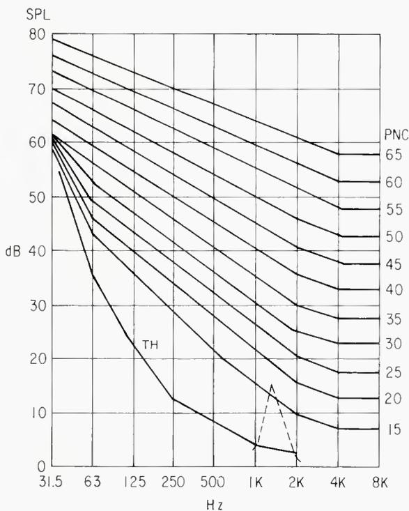
Figure 1. Preferred Noise Criteria (PNC) curves. Each curve is a code for specifying the noise level characteristic, or spectrum, of the noise in rooms. TH is the threshold of hearing for continuous noise fields. SPL is sound pressure level in decibels relative to 0.0002 microbars.
