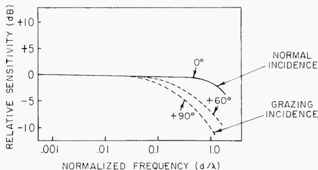
Figure 7. Perpendicular (zero degree) incidence and off-axis frequency response characteristics of a typical free-field microphone.
