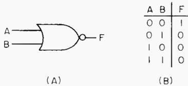
Figure 5. The NOR gate. (A) NOR gate logic symbol. (B) Truth table for NOR gate.
