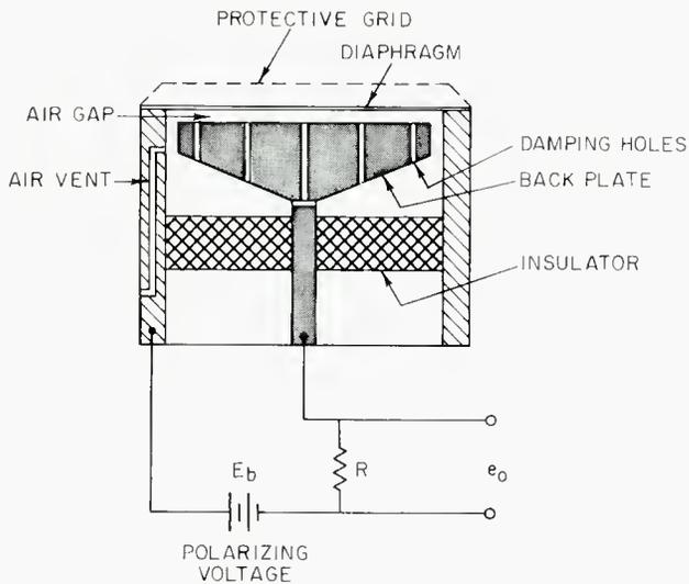
Figure 2. Schematic view of an air-condenser microphone.
