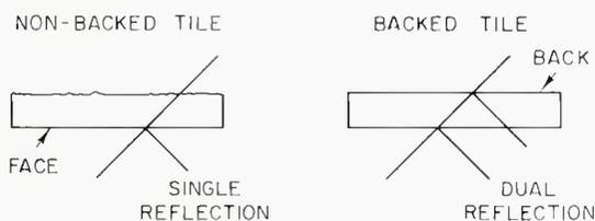
The efficiency of ceiling tiles varies. At times, compromises must be made because of cost. For example, one-inch backed ceiling board will transmit less signal into the plenum space and therefore more reflected signal into an adjacent work zone than thicker tile. But one-inch backed ceiling board may be considered desirable because it is economical. This is the type of tradeoff which often takes place in the extensive consideration of an open-office planning technique.
