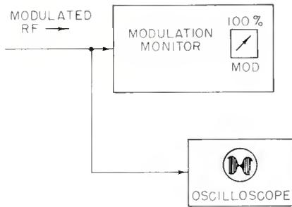
Check the accuracy of the modulation meter with an oscilloscope.
