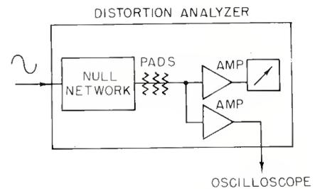
Basic modern analyzers null the fundamental tone and measure what remains as distortion.
