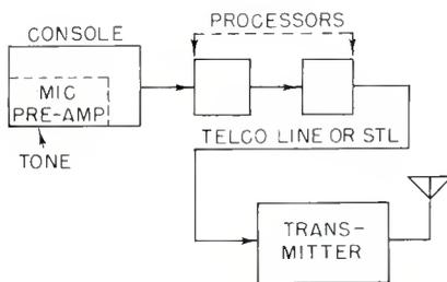
The basic chain is measured. Disable the AGC and other processing units, and make sure that the load on the transmitter is the antenna system.
