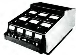
● With a cassette master and five slaves, the DP-4050-CCF in-cassette duplicator provides an 8:1 duplicating speed ratio. Cassette formats duplicated are:  $\frac{1}{4}$  or  $\frac{1}{2}$  track mono, or  $\frac{1}{4}$  track stereo, with all tracks recorded in one pass. The unit employs ferrite heads, and each plug-in slave unit is completely independent of the others, with its own servo-controlled capstan motor.
