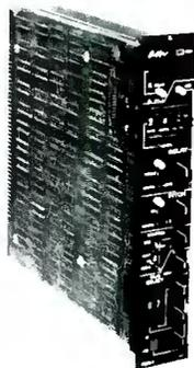
● Signal processing is featured in this month's **db**, and art director Bob Laurie shows us two views of one of the latest-generation devices: Audio Machinery's Shared Access Memory System. In the background, we see the art work for one of the p.c. boards in SAMS' mainframe computer system, where the system's microprocessor lives. Up front, one of the pitch/delay modules. For more details, see Michael Tapes' feature story in this issue.
