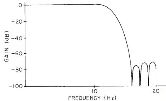
Figure 4. Frequency response of a 32-tap low-pass filter.
