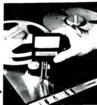
The Tentel tape tension gage is designed to diagnose problems in your magnetic tape equipment. Throw away your fish scales (or put them in your tackle box where they belong). The TENTELOMETER will measure tape tension while your transport is in operation, so you can "see" how your transport is handling your tape . . . smooth, proper tension for quality recording? or oscillating high or low tensions causing pitch problems, wow and flutter?
