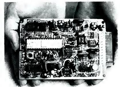
● The model 20, an LSI-based audio pitch shift module, produces off-speed audio intelligibility over a range from  $\frac{1}{2}$  to  $2\frac{1}{2}$  times normal sound speed. The unit offers a 100 to 5000 Hz  $+0/-3$  dB frequency response, a dynamic range greater than 56 dB, and 0.6 per cent total distortion and noise.
