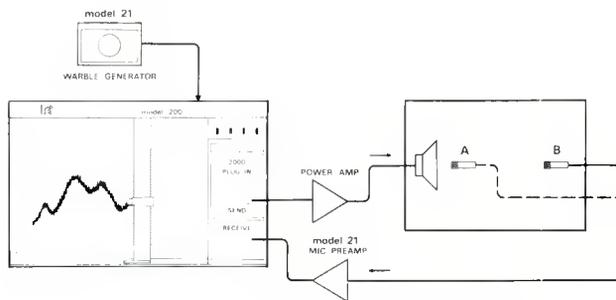
Figure 7. Acoustic frequency response measurement with warbled sine wave sweep.
