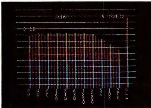
changing the measured value. In Badap 1, the peak value is a word in memory, and it will remain there, unchanged, until the memory is erased or the machine unplugged.
