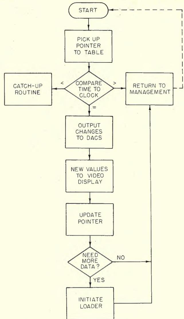
Figure 3. Flowchart of program section for playback.
