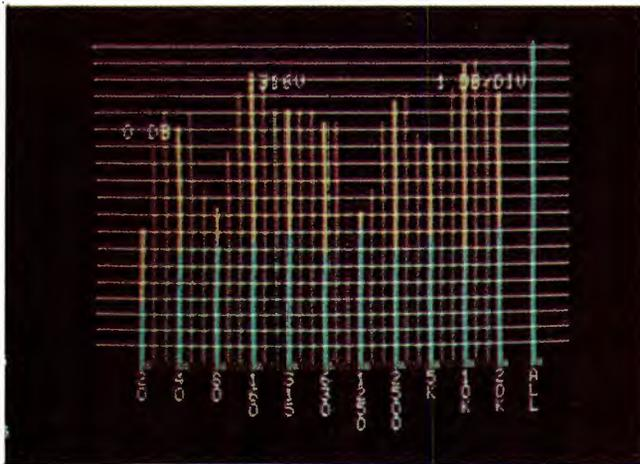
Figure 3. Response of a speaker before room equalization (yellow) and after (green).
