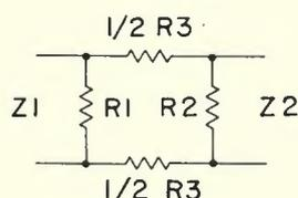
$$\begin{aligned} R_3 &= \frac{N-1}{2} \sqrt{\frac{Z_1 Z_2}{N}} \\ \frac{1}{R_1} &= \frac{1}{Z_1} \left( \frac{N+1}{N-1} \right) - \frac{1}{R_3} \\ \frac{1}{R_2} &= \frac{1}{Z_2} \left( \frac{N+1}{N-1} \right) - \frac{1}{R_3} \end{aligned}$$
