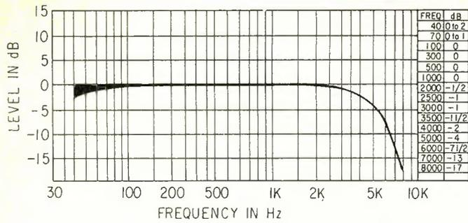
Figure 2. Motion Picture Research Council's standard electrical characteristics for Altec Lansing's Voice of the Theatre Systems. Electrical run, measured at the output of the power amplifier with a resistance equivalent to the speaker network load using the Research Council Standard Multi-frequency Test Film, Altec or RCA Test Film.
