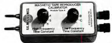
This is induction loop equipment of laboratory quality for primary standardization of tape recorders and tapes. Send for detailed information, prices and formats.
