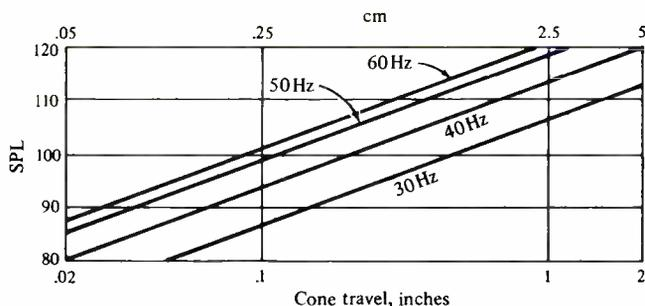
Figure 5. The required cone travel,  $D$ , of a 16-inch diameter loud-speaker cone from its mid or rest position at the indicated frequencies to generate various sound pressure levels, SPL, at a distance of 10 feet (3.05 m).
