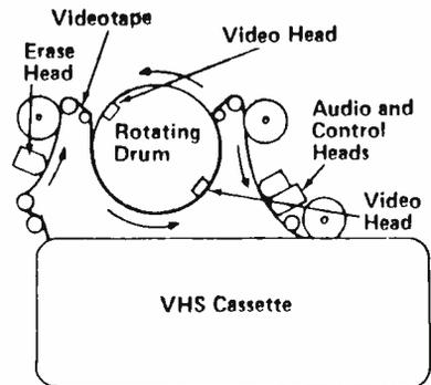
Although Beta and VHS Systems employ different tape loading systems, both use stationary audio recording and playback heads.
