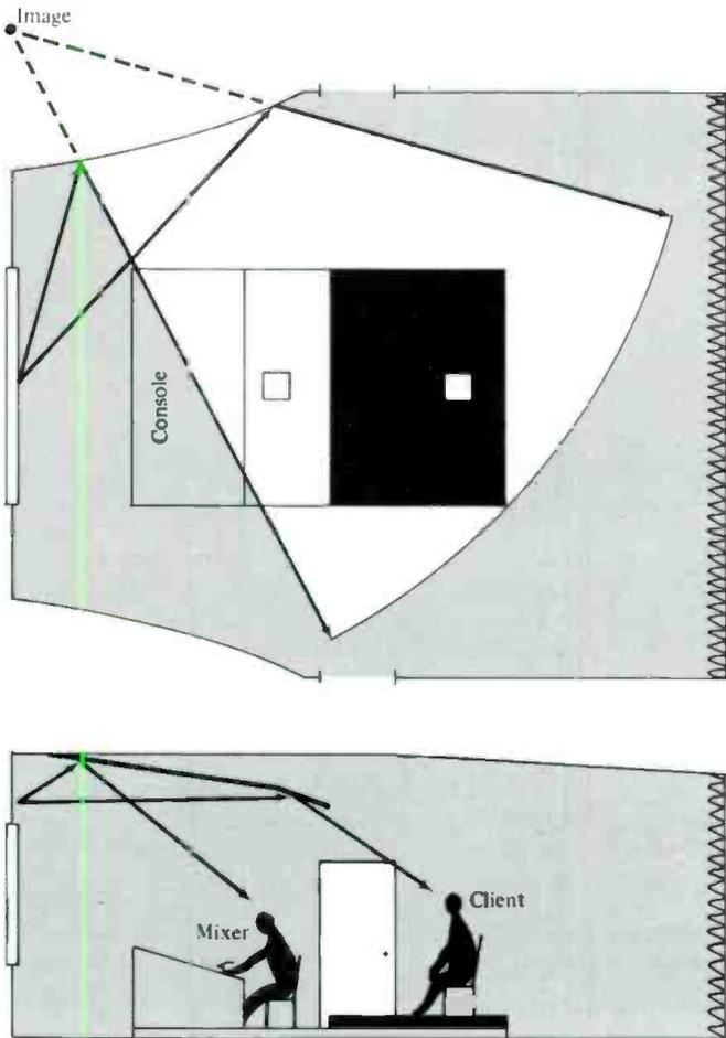
Figure 8. Recommended plan view and elevation for a control room of 5000 ft<sup>2</sup>.
