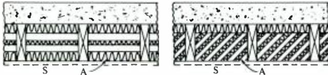
Figure 2. Anechoic treatments for the rear wall of the control room. A decorative screen (e.g., loudspeaker grill cloth) protects the 2 inch (5 cm) thick sound-absorbent fiberglass boards.
