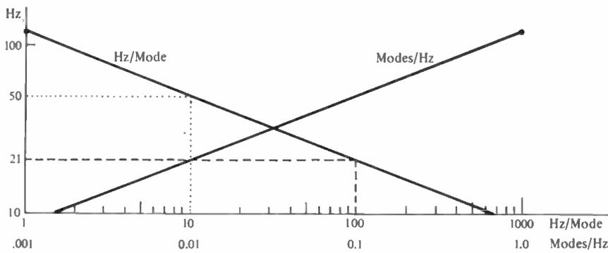
Figure 1. The average frequency space between modes (Hz/mode) for a control room of 5000 ft<sup>3</sup> volume, as a function of frequency. For example, at 50 Hz, a frequency space of 10 Hz exists between modes (dotted line). At 21 Hz, the modes are 100 Hz apart (dashed line).
