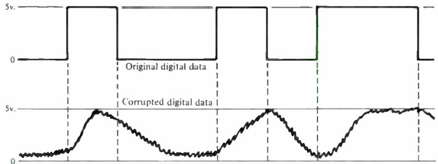
Figure 2. A digital waveform, before and after transmission over a noisy medium.
