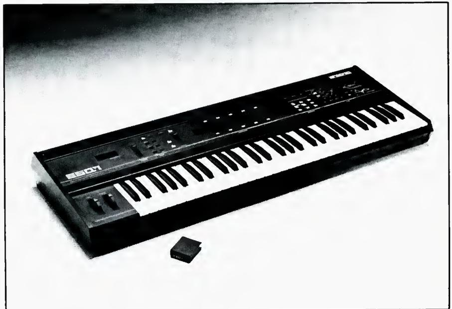
quencer with 2400 note internal storage (expandable to 10,000 notes) and 8 discrete tracks—each with separate program and MIDI channels. Each track has 8 voices dynamically assigned. The sequencer also features a mixdown facility for balancing individual tracks, sync to tape selector, built-in metronome and autolocator, plus 30 separate sequences chainable into 10 songs. External storage of
