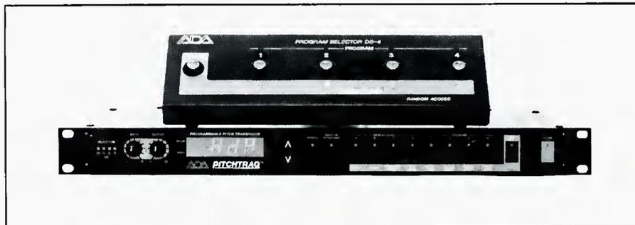
stage control. Other features include 15 kHz frequency response, an LED readout which displays pitch change in cents, ratio, or standard musical interval, and a self-diagnostic program
