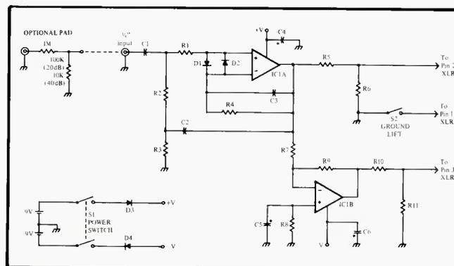
*Figure 1. Schematic of circuit for active direct box.*
