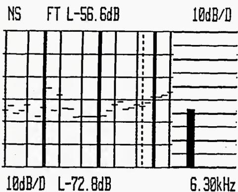
Figure 5B. Third order distortion vs. record level at 15 in.sec
