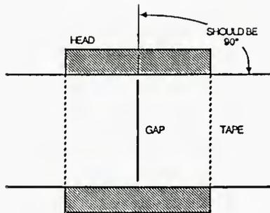
Figure 2. Azimuth alignment
