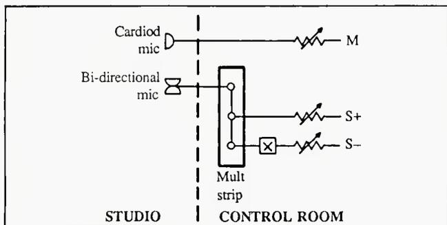
Figure 9. The setup for "coincident" or M/S mic-ing occasionally used by Estes as a point-source pickup for solo performers.
