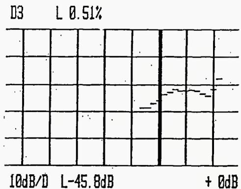
Figure 5A. Third order distortion vs. record level at 15 in.sec
