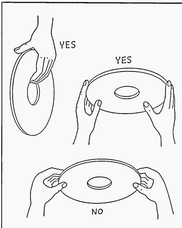
Figure 2. Handling tape reels.
