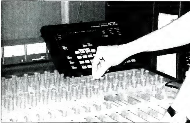
Figure 2. The Tascam M-520 with the Fostex 4035 Synchronizer in studio A.
