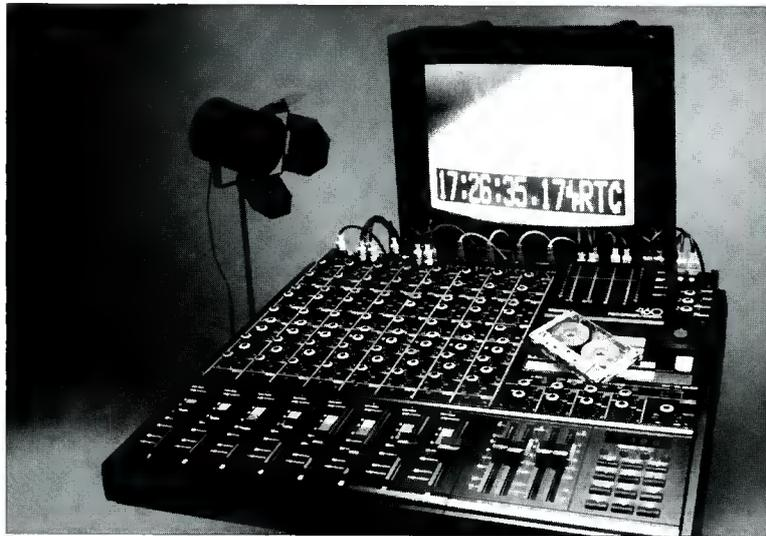
● The Fostex 460 is the company's top-of-the-line recorder/mixer. It includes a 4-track cassette recorder built into a complete 8-input mixer.
