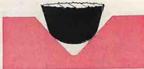
Conventional rounded stylus touches groove only tangentially at two points, resulting in enormous contact pressures. Even a light-weight pickup exerts point pressure of many tons per square inch.
