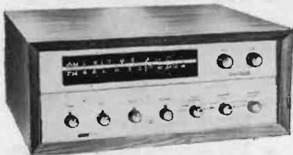
FM sensitivity is 3.5 uv for 30 db quieting (2.5 uv for 20 db), the bandwidth is 240 kc at the 6 db points, the circuit features AFC, a Foster-Seeley discriminator
