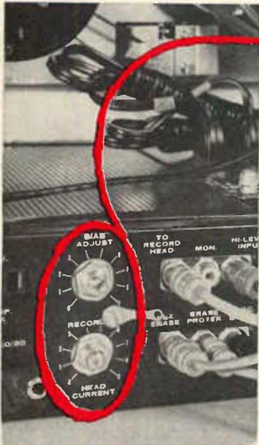
**BIAS ADJUSTMENT** enables the technically adept user to vary the amount of bias current for optimum performance with various types of tape. The rear apron of the Viking Stereo Compact has slotted control shafts for adjusting both the erase and the record current.
