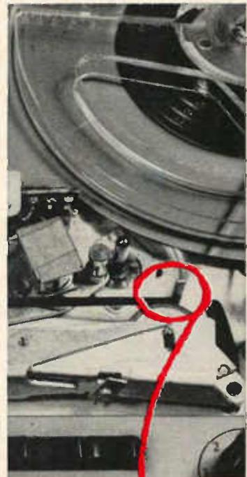
**TAPE LIFTERS** hold the tape away from the head surfaces during rewind and fast forward. The Tandberg Model 6 employs this type of mechanism.
