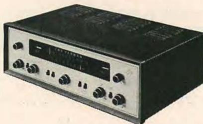
magnetic phono input and 53 db below full output on the tape channel. Channel separation is better than 42 db at 1000 cps. In addition to conventional rumble and scratch filters, a subsonic filter is included to provide sharp roll-off below
