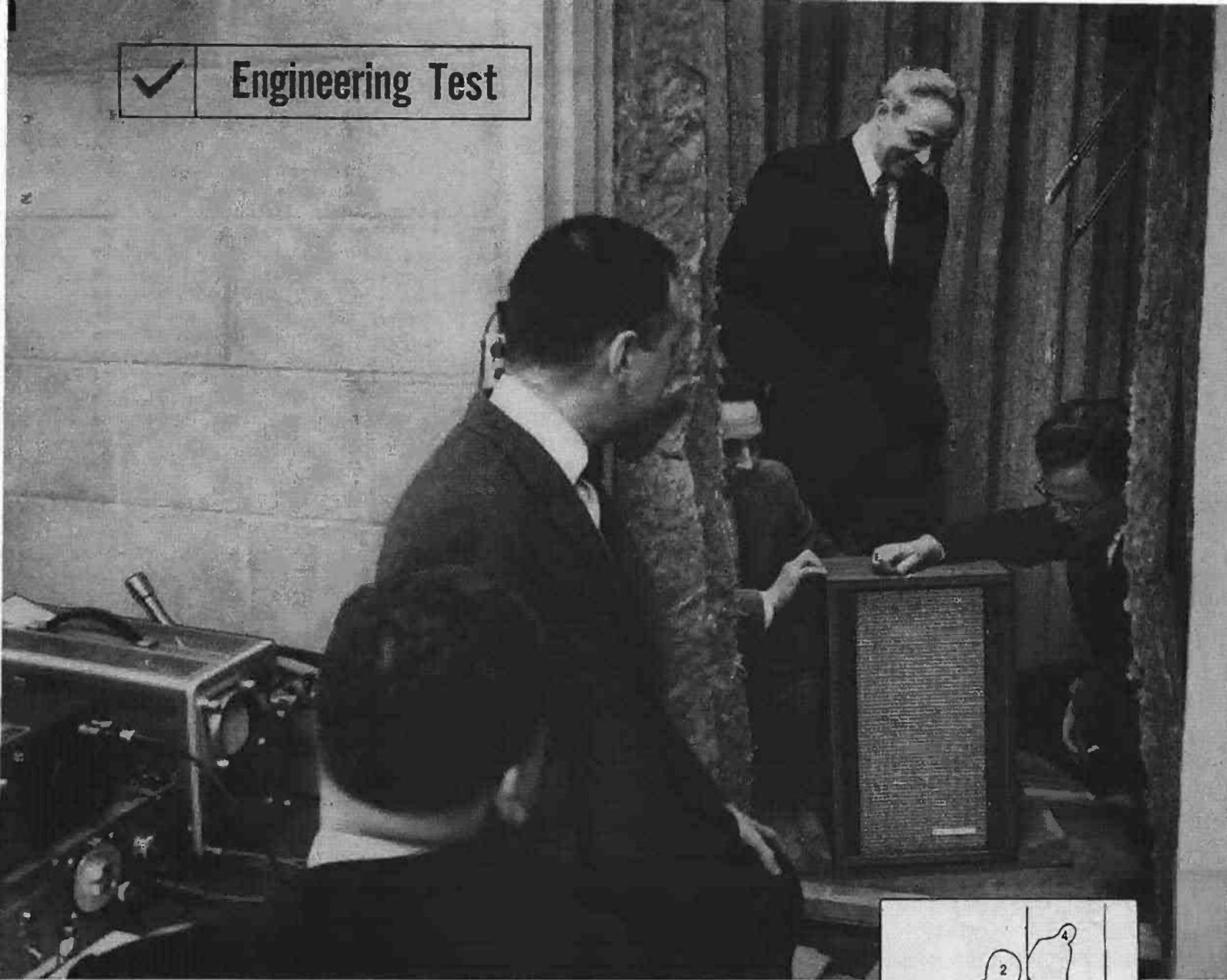
Scientists watch while Peter Globo, Speaker Development Engineer, makes exacting measurements on the new H. H. Scott speaker in anechoic chamber.
