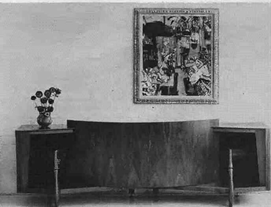
*The curved front of the James B. Lansing Paragon serves as a reflecting surface for two midrange horns, visible at each side. Woofer and tweeters are recessed at opposite ends of the enclosure.*
