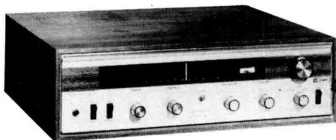
the receiver's features are a center-of-channel tuning meter, a speaker-muting switch, a front-panel headphone jack, a tape-monitor switch, and a built-in FM dipole antenna. FM tuner specifications include a sensitivity of 3 microvolts (IHF), 30 db of stereo separation, and 1 per cent harmonic distortion.
