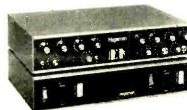
controls. There are also switches for input selection, mode, loudness, and a front-panel stereo-headphone jack. Between the two modules is a power supply for both, with three rear-mounted a.c. convenience outlets, two of them switched. The signal-to-noise ratio for the preamplifier module is 69 dB (phono input), and 90 dB for the control module (high-level inputs).
