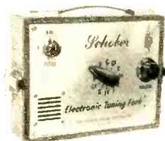
● **Schober** is marketing the Electronic Tuning Fork, a fully transistorized tuning device with built-in speaker that provides any of the twelve tones from middle C to the B above, according to the setting of the front-panel selector switch. The frequency of the tones is based upon the International Standard Pitch (A = 440 Hz). A pitch control allows any of the frequencies to be varied over a
