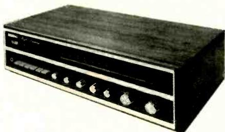
● THIS stereo receiver is the first of Harman-Kardon's import models that we have yet tested. Its styling is very much like that of their earlier receivers, with a black panel accented by contrasting polished metal knob caps and edge trim, and an opaque black dial face illuminated from the rear when the receiver is on. The 820's tuner section has a field-effect transistor (FET) front end, a four-gang tuning capacitor, and integrated circuits (IC's) and crystal filters in the i.f. amplifiers.
