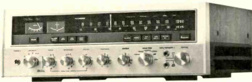
**1 Ultrasensitive FM Front End** Two RF amplifiers and one mixer amplifier use three costly, low-noise, dual-gated metal-oxide silicon field-effect transistors (3 MOSFET's) and a 4-gang frequency-linear tuning capacitor. These combine to give the EIGHT its great edge in such areas as FM intermodulation distortion, sensitivity (1.7 microvolts IHF), signal-to-noise (better than 65 db) and image-frequency, IF and spurious-response rejection (all better than 100 db).
