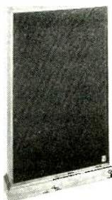
● FAIRFAX's top-of-line speaker system is a four-way twelve-driver design called the "Wall of Sound." The tall, shallow enclosure (52 x 30 x 6 $\frac{1}{2}$  inches) is partitioned into various acoustical paths and chambers, terminating in ports for the woofers. Six 8-inch woofers handle the frequencies up to 1,500 Hz, where two 5-inch mid-range drivers take over to extend response to 5,500 Hz. The upper mid-range (to 9,000 Hz) is handled by two 3 $\frac{1}{2}$ -inch cone drivers. The frequen-
