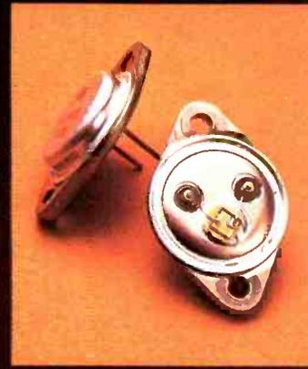
**Darlington Fully Complementary Monolithic Output Transistors.** These components actually house two devices—the driver transistor as well as the output transistor—assuring optimum match, a simplified circuit design and better reliability. It's expensive, but the result is better power bandwidth and improved high frequency performance.
