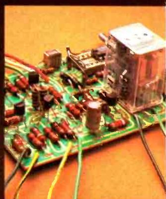
**Exclusive Impedance-Sensing Overload Protection Circuit.** [Patent applied for] New "ISOP" circuit senses the exact impedance condition of speaker load as well voltage to it; offers double protection to output devices and speakers.
