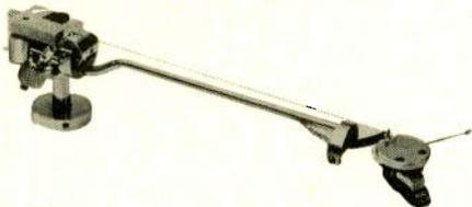
● TRANSCRIPTORS (Ireland) Limited is importing the "Vestigal" Tone Arm, a new design employing a vertical pivot assembly located very close to the phono cartridge to reduce effective tone-arm mass in the vertical direction as
