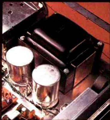
**The Power Supply.** The S7900A/S8900A uses an extremely well regulated power supply. The heart of it is a massive power transformer employing very high purity iron core material and heavy gauge copper wire for increased operating efficiency and improved voltage regulation. Two large 7000 mfd electrolytic capacitors insure the maximum in clean, well-regulated, low frequency audio output.
