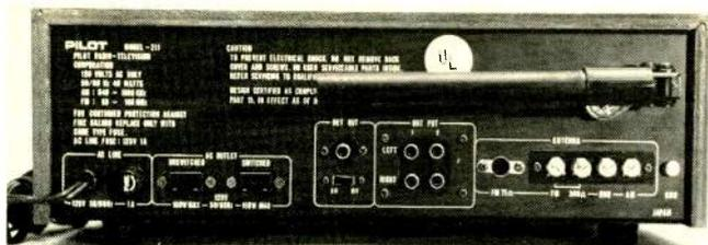
The Pilot 211 has a rather elaborately equipped rear panel. There are two sets of audio outputs, plus an FM DET jack (in anticipation of four-channel FM), and two a.c.-line convenience sockets.
