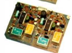
AN-2016 SPECIFICATIONS — PREAMPLIFIER — Frequency Response: 10-30,000 Hz. -0.5 dB. Total Harmonic Distortion: 0.05%. Intermodulation Distortion: 0.05% Hum and Noise: phono. -75 dB (ref. 10 mV input); hi-level. -80 dB (ref. 0.25V input). — FM — Sensitivity: 1.7  $\mu$ V. Total Harmonic Distortion: less than 0.3%. Alternate Channel Selectivity: greater than 100 dB. Capture Ratio:
