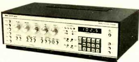
bringing in all stations along the way or, if desired, only the stereo stations. The tuned frequency is indicated by a brightly lit light-emitting diode (LED) digital display; additional LED's show signal strength, register the presence of multipath, and indicate the operating mode of the tuner.
