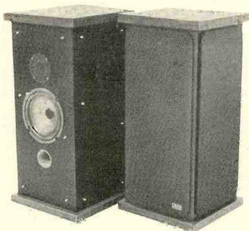
**A**VID's Model 101 is a floor-standing speaker system that is roughly columnar in shape. The cabinet's top and bottom are made of walnut-finish wood and three sides are covered by removable brown grille cloths. The black rear surface of the cabinet is its only unfinished side. The speaker terminals are located under the base, so that connecting wires enter at floor level.
