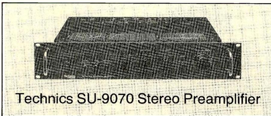
TECHNICS refers to their SU-9070 stereo preamplifier as a "flat" amplifier. This is a particularly apt description, since the SU-9070 is not only physically "flat" (built in the currently popular low-profile format) but is also as electrically flat as one could desire. It is, in addition, a d.c. amplifier, with no capacitors whatever in the signal path from its high-level inputs to the outputs. However, a second set of output jacks is available with capacitive output coupling.
