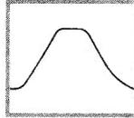
*Pulse waveform response of a conventional amplifier.*
