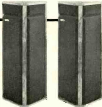
The ALLISON:ONE® Room Matched® loudspeaker system was introduced in 1974. It was the first direct-radiator system ever designed to use room-boundary reflections constructively, so that flat acoustic power could be radiated into a listening room throughout the full frequency range.
