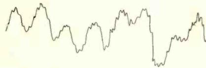
This same curve might also be an audio waveform as displayed on an oscilloscope screen. In this interpretation, time runs from left to right and the height of the curve represents the audio voltage at any instant. High frequencies (the narrow peaks) are undulations that occupy short time periods; low frequencies take longer and appear wider. If we want someone to reproduce this tracing, what kind of measurements should be made and sent?
