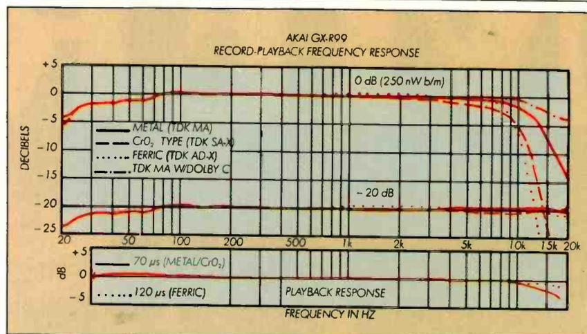
The upper curves indicate overall record-playback response at the manufacturer's indicated 0-dB recording level using the tapes designated on the graph. In the center are the same measurements recorded at -20 dB relative to the upper curves, a level used for frequency-response measurements. Bottom curves show playback response with calibrated test tapes and indicate performance with prerecorded tapes.
