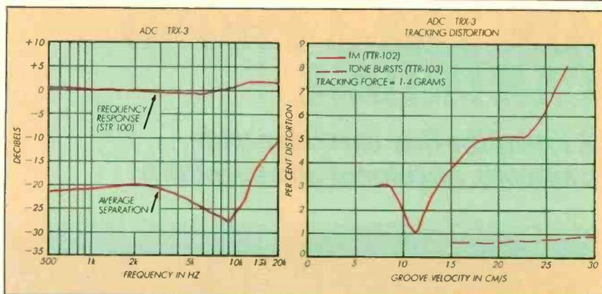
In the graph at the left, the upper curve represents the frequency response of the cartridge. The distance between it and the lower curve is the average separation. The right graph shows the tracking distortion with various test signals.
