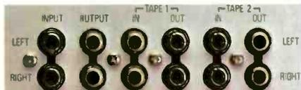
And, look at this. There are two tape inputs and outputs, so you can dub from tape deck A to B, or make two tapes at once with or without equalization.
