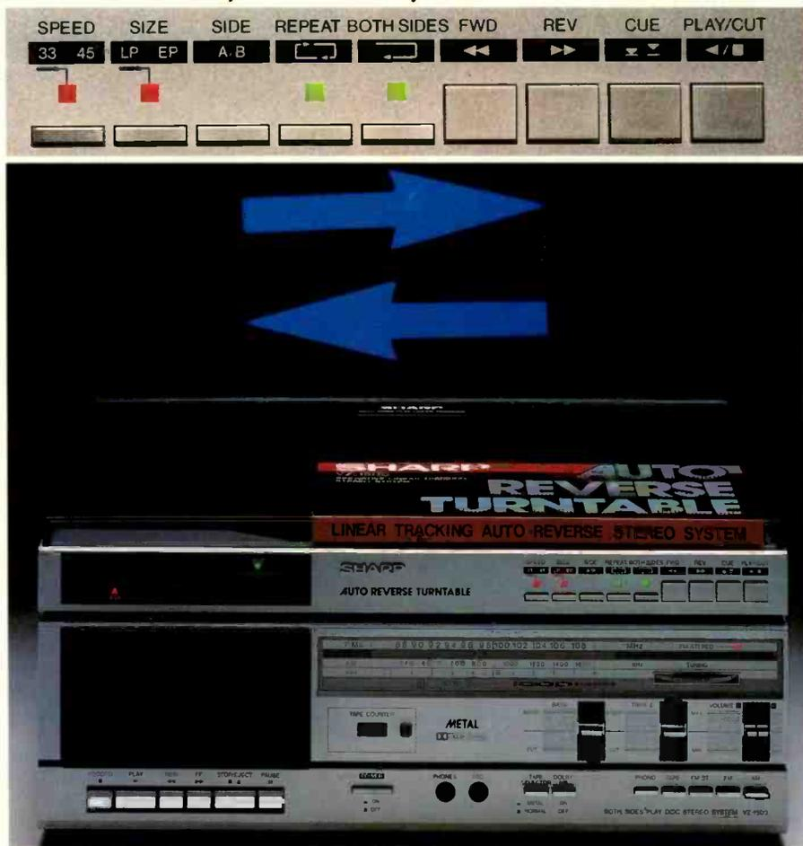
And, while most of the space here has been devoted to the revolutionary turntable, let's not forget the cassette deck. It's really a component quality, soft-touch deck. It has a hard permalloy head for high quality recording.
