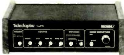
duces high-frequency hiss and noise. As many as three stereo or four mono inputs can be routed through the Teledapter. Input impedance is rated at 48,000 ohms and output impedance at 100 ohms. There is both a 75-ohm video-monitor output and a built-in Channel 3/4 modulator. The unit measures 8½ x 2½ x 7 inches. Price: \$149.95. Rhoades, Dept. SR, P.O. Box 1052, Columbia, TN 38401.
