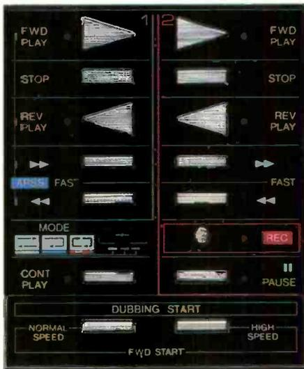
You can set the decks to play one way only, both sides of one cassette or both sides of both cassettes. There's a built-in automatic recording level circuit for perfect dubs every time.
