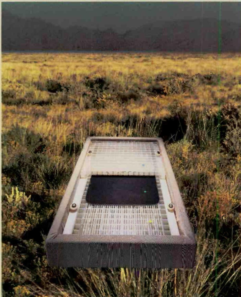
*A demonstrator panel for Acoustat electrostatic speakers shows a black, conductive Mylar diaphragm sandwiched between two electrically charged grids. An audio signal fed to the diaphragm causes it to oscillate back and forth, moving air on both sides of the panel.*
