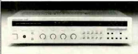
deliver 45 watts per channel into 8 ohms from 20 to 20,000 Hz with 0.08 percent total harmonic distortion. High-current capability is given as 20 amperes. There are eight station presets and two tape monitors with tape copy. The phono section has two RIAA equalization networks, one for low-frequency boost and high-frequency rolloff, the other to maintain the same low level of negative feedback at all frequencies from 20 to 20,000 Hz. Price: \$435.
