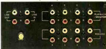
And 1 'Enhancer' can feed all your decks when you use its tape monitor circuit.
