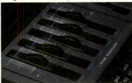
The 5 band EQ lets you sculpture the sound just the way you like it at 100hz, 330hz, 1,000hz, 3,300hz, and 10,000hz.
