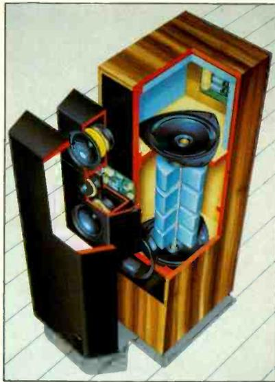
*This cutaway drawing shows the unusual construction of the KEF 104.2's bass system. The push-pull low-frequency drivers operate totally within the cabinet, their output reaching the outside via a large, front-panel port.*
