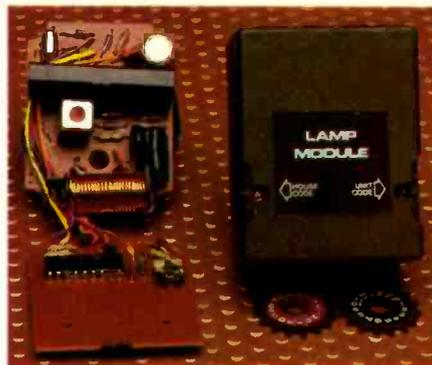
Each module has a rotary dial numbered from 1 to 16. Just dial in a number to match one of the 16 number buttons
