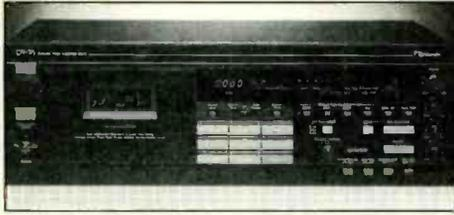
**N**AKAMICHI was the first company to produce a three-head cassette deck, and the CR-7A continues in Nakamichi's tradition of innovation. A four-motor deck with closed-loop dual-capstan drive, the CR-7A has such additional refinements as user-adjustable playback azimuth alignment and a sixty-four-step tape-optimization system controlled by a 6-bit microprocessor.
