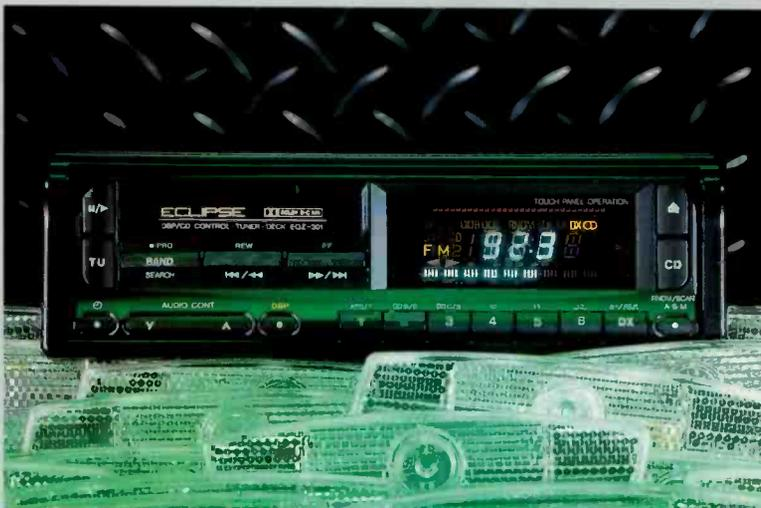
The EQS-1001 was solid on the test bench. Frequency response was nearly flat, and the signal-to-noise ratio was impressive. Distortion was low at 0 dB and remained relatively low at -20 dB. Interchannel phase error was negligible. Signal-path linearity deviated by only a tiny amount at the -70-dB test level.
