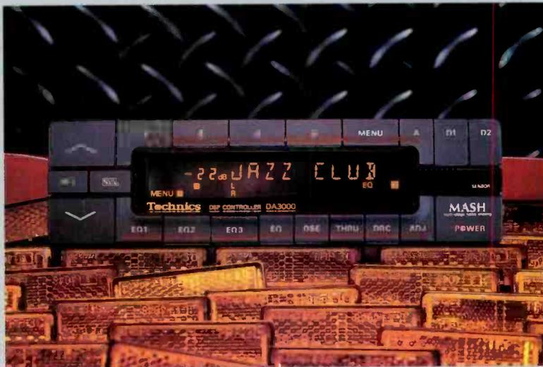
The DA3000 delivered generally good numbers on the test bench. Frequency response was down only slightly at 20,000 Hz. Channel separation was more than adequate, and the signal-to-noise ratio was respectable. Distortion was low at 0 dB but rose somewhat at -20 dB, and conversion linearity was good.
