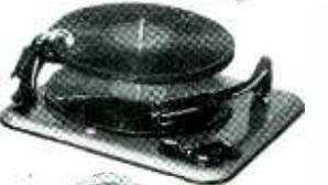
**G.I. 3-SPEED CHANGER.** These units automatically play all 3 sizes of records—7", 10" and 12". Motor provides 3 constant speeds— $33\frac{1}{3}$ , 45 and 78 rpm. Tone arm uses crystal cartridge with single .002" needle to play both standard and microgroove records. Size:  $12\frac{3}{4} \times 12 \times 5\frac{7}{16}$ ". Requires 4-1/16" above  $3\frac{1}{2}$ " below. Wt., 12 lbs.
