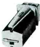
One unit with two replaceable styli and one pressure (8½ grams) for all three: 33⅓, 45, and 78 rpm. Provides excellent coupling between styli and groove with high stylus compliance and minimum mass. Response from 20 to over 10,000 cps. with output about 20 millivolts. Practically no needle-talk.
