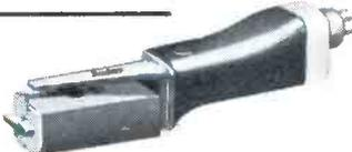
Plug-in magnetic head for Garrard record changer. Uses Audax polyphase principal. A simple twist brings either the standard or microgroove stylus into play. Sapphire stylii. Fine reproduction. Only 6-8 grams stylus point pressure.
