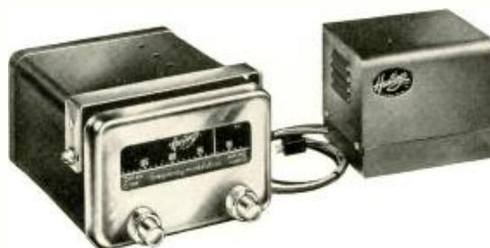
Mobile FM tuner with optional combined amplifier-power supply.
