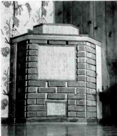
*The permanent-type speaker enclosure at the left houses a 12-in. Wharfedale woofer; a cone tweeter in the little box above points upward. A. J. Whitfield made the Briggs-designed system as part of a music installation for George Pears in Victoria, British Columbia. He describes the sound as "well-balanced, very satisfactory." Below is a California custom installation by Kierulff Sound Corporation of Los Angeles; the door in the left foreground is part of a matching TV console.*
