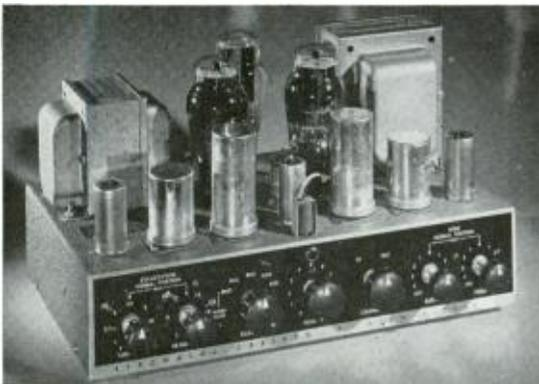
*The AR-420 has a complete but simple preamp-control section.*
