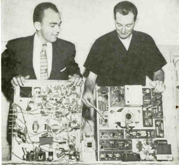
No more "jungle" of wires. Chief Engineer Fred Miller (right) makes a side-by-side comparison of a Walsco PC-9 (right) with a conventional, complicated chassis. Bob Mueller, Walsco Sales Manager, observes simplicity of vertically mounted, printed circuit design.
