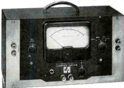
Tape recorders produce flutter and consequent frequency modulation noise for many reasons — and it is impossible to perform the adjustments necessary to maintain high quality reproduction without a flutter meter.
