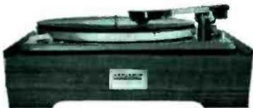
**New Miracord 18H** single record play turntable operates manually or automatically. Offers new cueing record band selector. Gently lowers arm and sets stylus in desired band or groove. Includes famous Miracord features: automatic pushbutton controls, Papst hysteresis-synchronous motor, heavy balanced turntable platter, transcription arm, four speeds.
