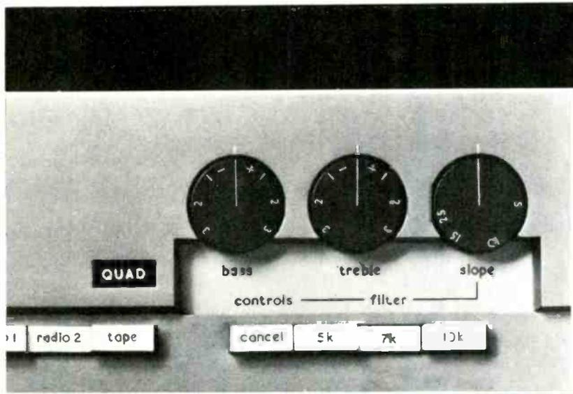
Set up a QUAD 33 with +1 on the treble control, and you will obtain a response precisely defined; readily and accurately repeatable. This response has a shape rather different from most run of the mill tone controls and there are, as you may guess, good reasons for this.
