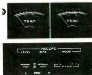
All-tape biasing and monitoring with Switchable Bias Control and Expanded VU Metering System for maximum performance with standard or low-noise/high-output tapes: the expanded-scale VU meter lets you read +3 dB at the "O" position, so your readings have a common reference point for either kind of tape. Completing this system is a convenient Tape/Source monitor that selects the signal displayed on the VU meters, and also available at the headphone output jack.
