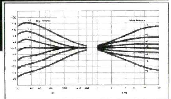
*The Bass and Treble Controls provide smooth and independent adjustment of the response to suit programme or environment*
