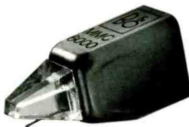
An integrated system, the MMC 6000 leaves the factory as a sealed unit, a non-replaceable stylus assembly integrated with the coils, magnet, and output terminals. This significant departure from traditional "two piece" cartridge design represents an absolute, no compromise approach to optimum CD-4 reproduction. The integrated approach allowed Bang & Olufsen engineers to greatly reduce the effective tip mass, the size and mass of the cantilever, and the transducing elements of the MMC 6000.
